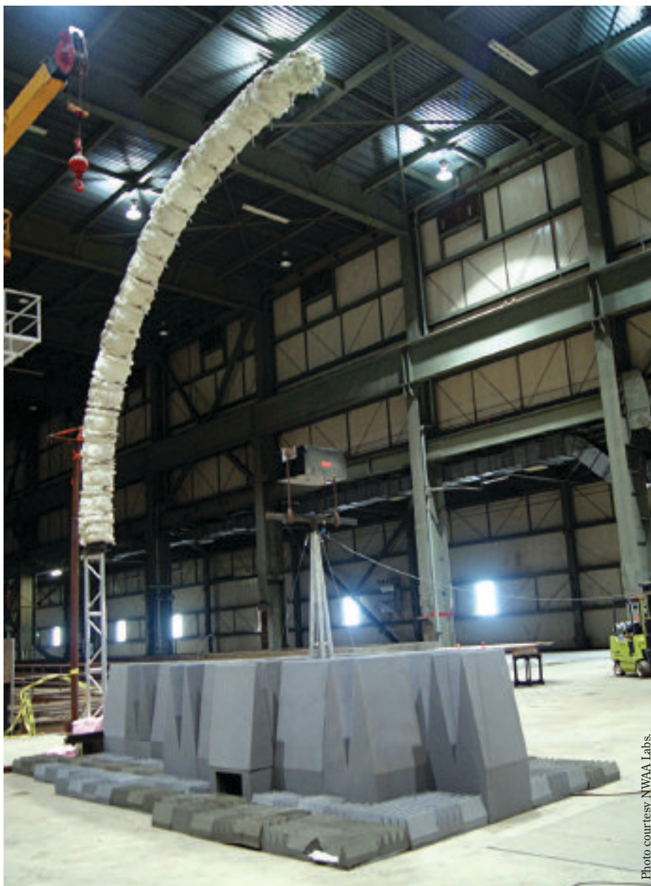
The massive diffuser-testing rig at NWAA Labs in Elma WA is housed in a giant room that is larger than a football field.
